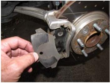
6. Remove the disc pad backing plate (inner and outer).
