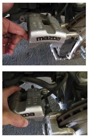
3. Swing the caliper up and ease the upper slider pin out of the mount bracket.
