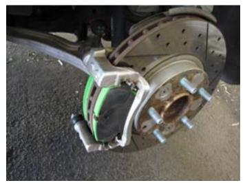
10. Put a <u>very light</u> coating of brake grease on the inside of the backing plates and position them on the back of the new pads.
