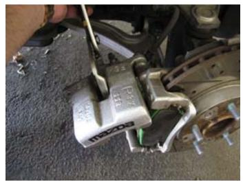
11. Place the upper slider pin back in the mount bracket upper hole and use the channel lock pliers to press the piston back into the caliper body so the caliper will clear the new disc pads. Make sure the brake fluid does not overflow the master cylinder. Use turkey baster to remove brake fluid as necessary.
