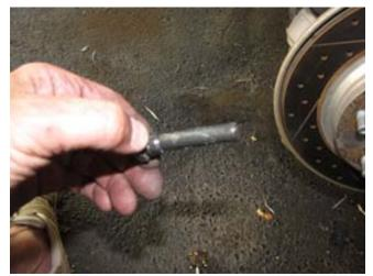
4. Remove the upper and lower slider pins from the caliper mount bracket and lubricate.
