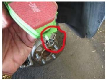
8. Pay attention to the "squealer" wear indicator clip and replace on the proper pad. Mine was on the inside pad, passenger side.
