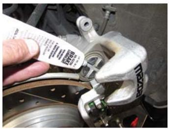
13. Lubricate the contact area of the caliper piston.
