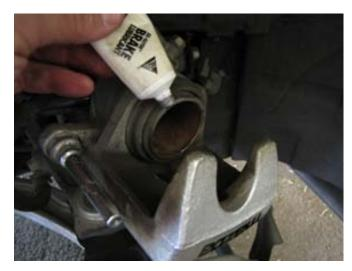
5. Lubricate the contact area of the caliper piston.
